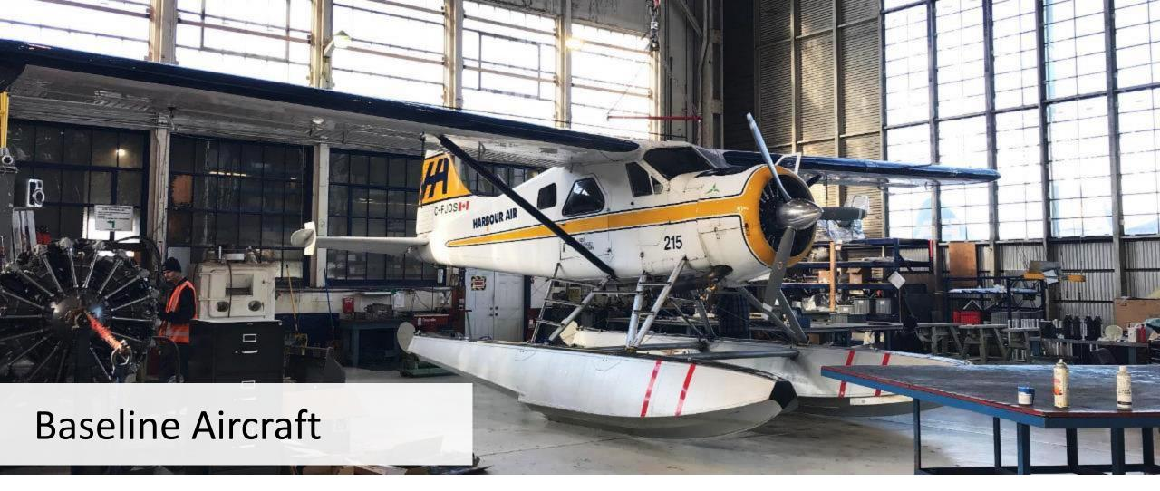
Pilots: 1 Passengers: 6 MTOW: 5,600 lb Dimensions: 10m x 15m x 3m Cruise: 180 km/h (~100 KTS) PowerPlant: P&W R985 Max rated power: 450 hp **First Flight:** August 16<sup>th</sup>, 1947 **Production:** 1947 – 1965
